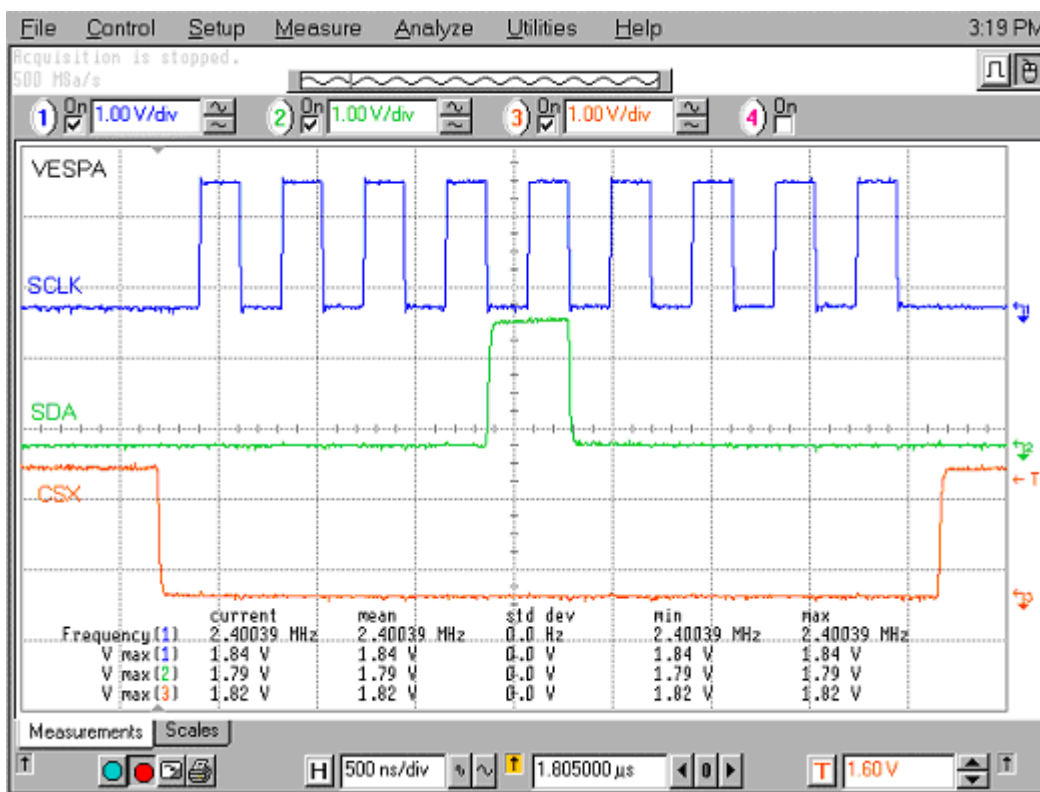
Figure 14: Waveform for the LCD Interface
